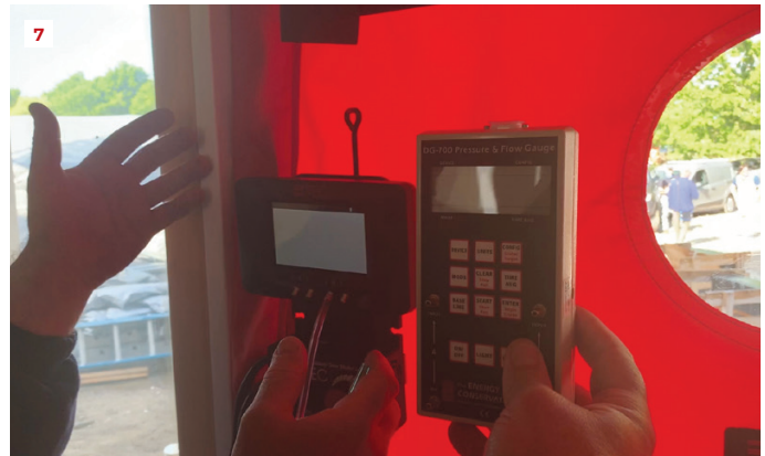
With the smoke test completed, the authors depressurized the home and performed a blower door test (6).
