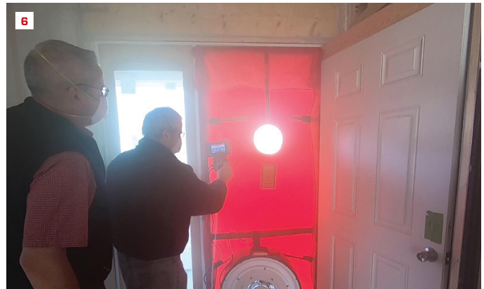
With the smoke test completed, the authors depressurized the home and performed a blower door test (6).
