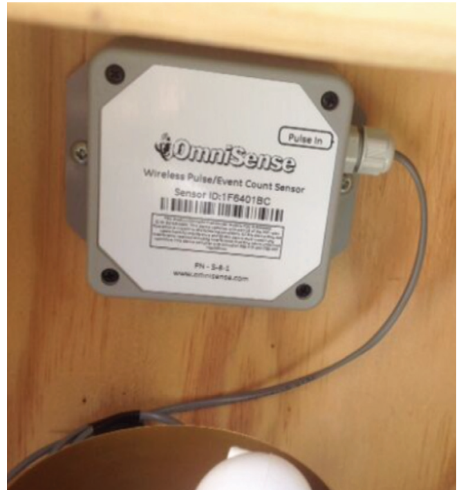
Lew Harriman and colleagues devised the system shown above to measure the water output of a house air conditioning and dehumidification system. Water emitted by the building's condensate drain filled a bucket, which tipped over when full (left); a pulse counter (right) counted the bucket tips, keeping a running total of the drain's performance.
