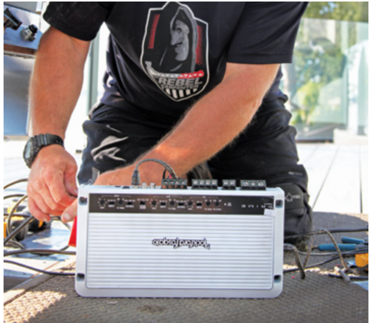
Figure 2. At the heart of the sound system is a Rockford Fosgate Prime M600 marine-grade 5-channel amplifier, paired with a matching Bluetooth receiver. Since the components operate on 12-volt DC power rather than 110-volt house current, a converter/charger sized to match the amp is also required to power the system.
