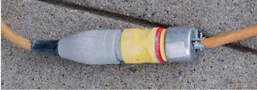
Figure 5. The Qwik-Lok fitting on the female end of this extension cord connects to the male end of the tool plug, eliminating the need to knot cords together.
