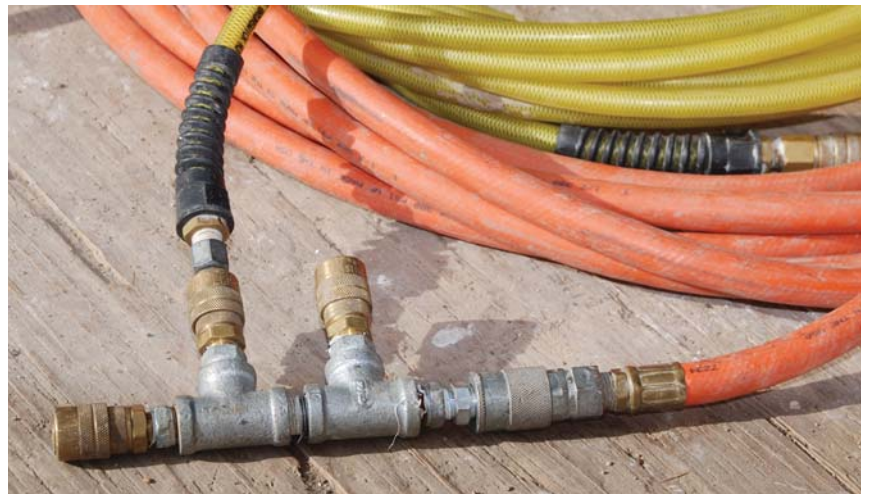
Figure 4. The author uses 1/2-inch rubber hose for main runs and branches off to individual tools with 3/8-inch polyurethane lines. He avoids using 1/4-inch hose because it's easily clogged by frost.
