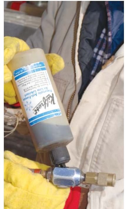
Figure 2. The author puts Kilfrost, a synthetic de-icer and lubricant, into an oiler at the end of a hose that will connect to a gun.
