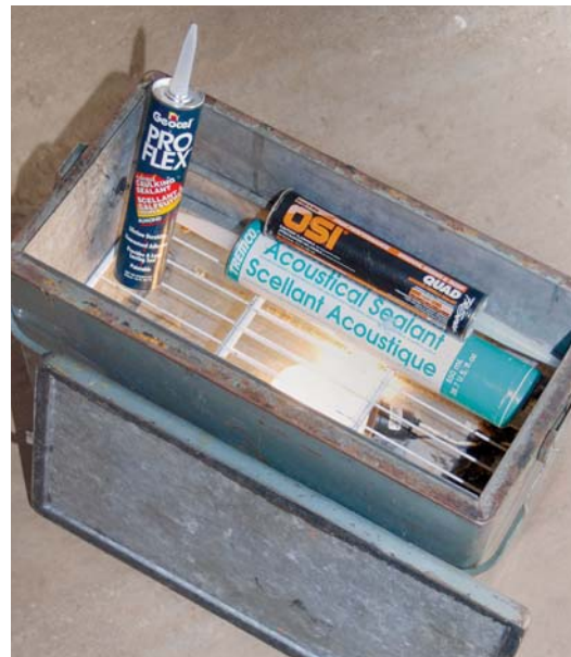
Figure 6. When the weather is cold, the author stores caulks and sealants in an old metal cooler heated by a light bulb. A rack keeps the tubes off the bulb.
