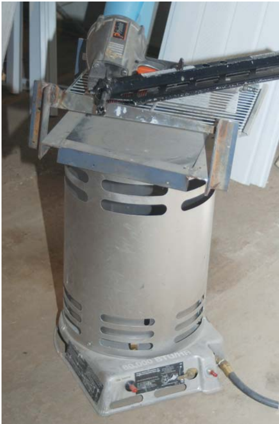
Figure 1. A homemade grille keeps tools far enough above the heater to ensure that they won't be overheated while they're being defrosted.
