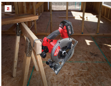
1. The 6 1/2-inch Milwaukee can cut through a 2-by at a 45-degree bevel. 2. Unlike the Makita, the Milwaukee has a built-in rafter hook. 3. The author did some serious framing using the 7 1/4-inch Makita, including trimming LVLs.
