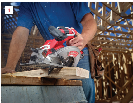
1. The 6 1/2-inch Milwaukee can cut through a 2-by at a 45-degree bevel. 2. Unlike the Makita, the Milwaukee has a built-in rafter hook. 3. The author did some serious framing using the 7 1/4-inch Makita, including trimming LVLs.
