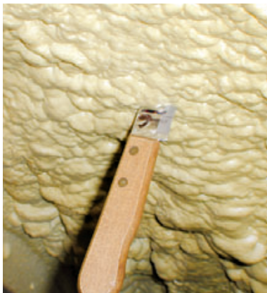
Figure 4. A cheap kitchen knife — with graduated inch markings added to the blade with a permanent marker — is a handy tool for cutting samples and confirming material thickness.
