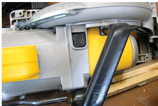
The DeWalt's blade-lock button is conveniently located, making blade changes a snap.
