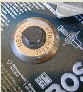
Bosch and several other manufacturers mark directional arrows on the left-hand-thread blade bolts.
