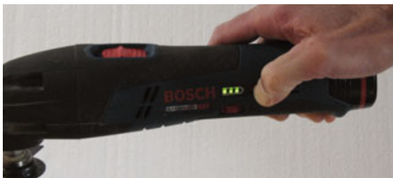
The Bosch PS50 shows its battery's charge level with the touch of a button.
