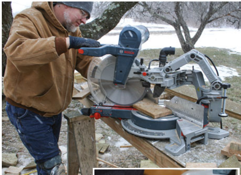
The GCM12SD glides back and forth on a set of knuckle joints. While most of the controls are up front on the swing-table handle, there are enough functions that actually reading the manual is a practical necessity. (The photo at right was shot by David Frane.)
