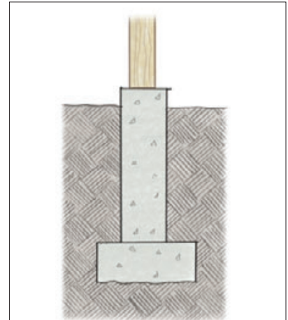
Figure 5. When larger loads dictate a large footing diameter, a pier/footing — a footing of the required thickness topped with a narrower concrete pier — is used instead of a large-diameter concrete column extending to grade.
