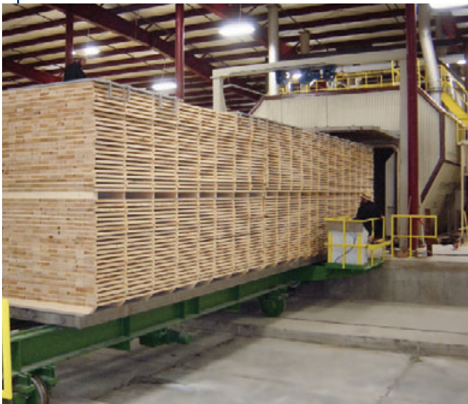
Figure 3. To minimize wood movement in the kiln, Bay Tree Technologies stickers and weights the lumber.
