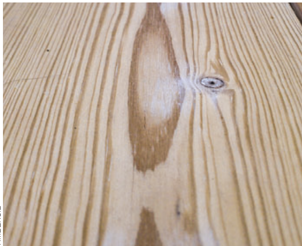
Figure 5. TimberSil preserves and stabilizes wood by infusing it with “liquid glass.”
