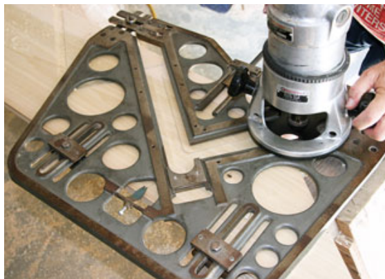
Figure 4. The stair template in this photo (left) provides precise control over the routing process but is no longer sold. In the past, the author made a throw-away version for each new job (below). The one shown is made from a scrap of cellular PVC panel, but plywood serves just as well.
