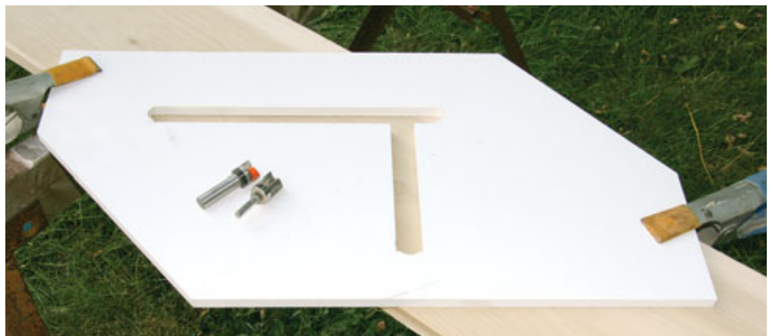
Figure 4. The stair template in this photo (left) provides precise control over the routing process but is no longer sold. In the past, the author made a throw-away version for each new job (below). The one shown is made from a scrap of cellular PVC panel, but plywood serves just as well.
