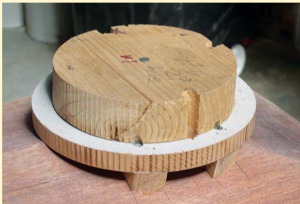
Figure 5. Here, bevel-edged mahogany planks for the railing cap are glued together with epoxy, the joint held snug with shipping tape until the adhesive cures (above). To create a flat bottom for mounting on the wall, a filler piece was added and bonded with more epoxy (right). Circular mounting blocks for the composite columns were installed in the shop (below); the lower disk matches the outside diameter while the upper receives screws driven through the column and concealed by decorative plinths. Note the weep holes for drainage and ventilation.
