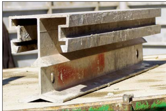
FIGURE 5. Special ledger cap forms are clipped to the top of the inside wall forms (above). Shoring beams of various lengths and widths integrate with the slab forms to allow for a range of floor sizes (left). Crews set slab form panels to span between the ledger forms and the shoring beams (below), creating the form system for a monolithic wall-and-slab pour.
