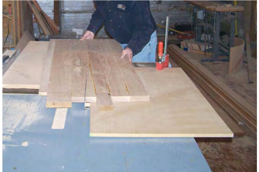
Figure 5. The author glues up blanks from \frac{5}{4} -inch stock, making them wide enough to cut two wedge-shaped treads with a tapering jig and long enough to allow for planer snipe. To make it easier to cut the mitered returns, 2-inch-wide nosings are fastened to the treads with pocket screws and glue.
