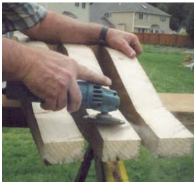
Figure 3. It's nearly impossible to cut thick stock perfectly, but a coarse abrasive disc makes quick work of the glitches.
