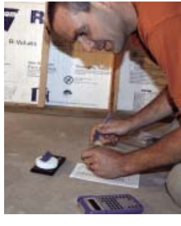
Figure 4. Some 60 to 72 hours after sealing the dome, the author slices it open and removes the container of calcium chloride (left). He then reweighs the container plus the tape that once sealed it (above left) and uses a formula provided by the manufacturer to calculate the moisture vapor emission rate — or MVER — of the slab (above right).
