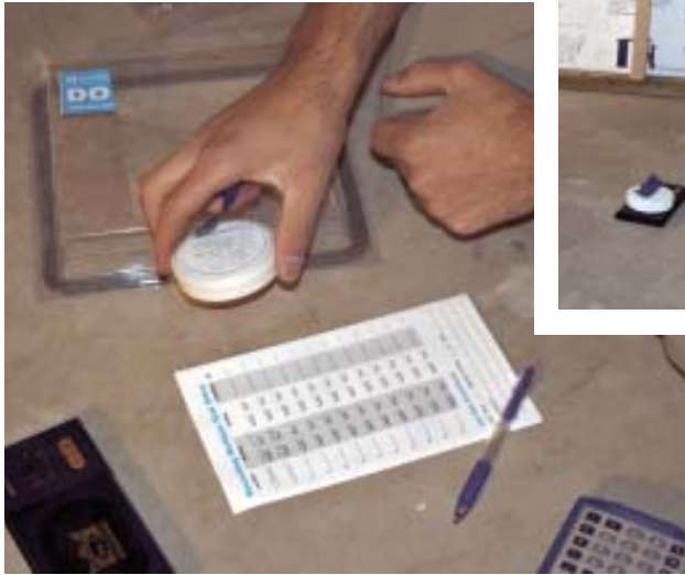
Figure 4. Some 60 to 72 hours after sealing the dome, the author slices it open and removes the container of calcium chloride (left). He then reweighs the container plus the tape that once sealed it (above left) and uses a formula provided by the manufacturer to calculate the moisture vapor emission rate — or MVER — of the slab (above right).
