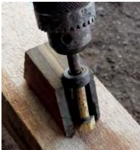
Figure 12. A long level on the tread noses establishes the stair pitch, and a Speed Square, held level, measures the stair angle (above). Use the angle to make a simple guide block for drilling cable holes in stair posts and newels (left).
