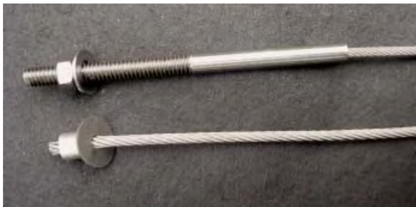
Figure 9. Studs and stops end the cable runs. Stops are simple aluminum rings that are swaged onto one end of the cable. Used with a washer, they resist the tension applied by the stud. The author has studs made locally from stainless steel rod; they're swaged to the cable and tightened with a nut.
