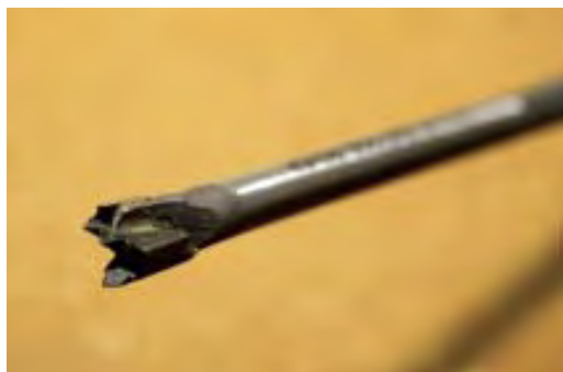
Figure 10. Curving holes are made possible with Rover bits by Bad Dog Tools.
