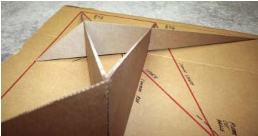
Figure 5. To develop the hip backing angle (angle LNM in the example), first draw a line perpendicular to the hip length extending to the base of the hip — from point J to point K. Next, draw a line from point K perpendicular to the hip run extending in both directions until it crosses the plate lines (LM). Then, using K as the pivot point, swing an arc from point J to the hip run — to point N in the example. Finally, draw lines from N to L and M; the resulting angle, illustrated in the cardboard model (photo, left), represents the top of the hip rafter.
