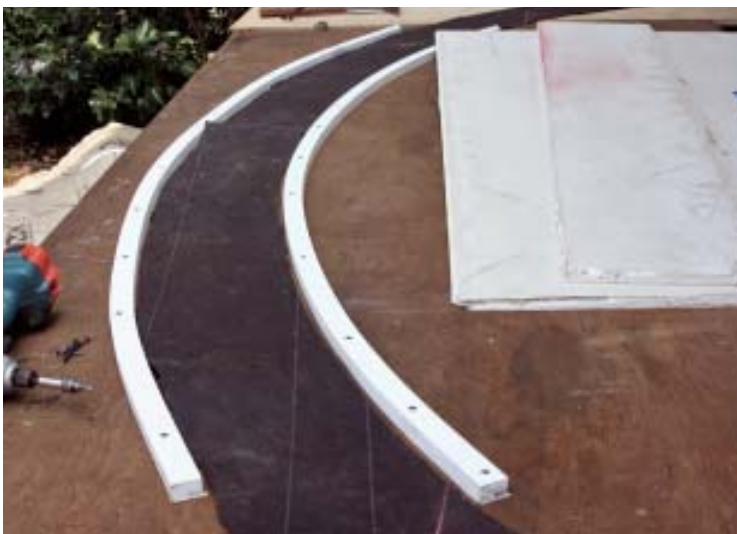
Figure 3. To make a form for the trim, 1-inch-wide PVC rippings are screwed to the worktable, with the felt-paper template serving as a guide (above). The PVC trim is warmed with heat blankets; scraps of drywall prevent heat loss and speed up the process (right).
