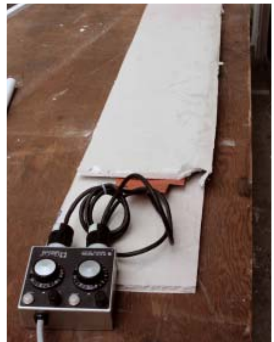
Figure 3. To make a form for the trim, 1-inch-wide PVC rippings are screwed to the worktable, with the felt-paper template serving as a guide (above). The PVC trim is warmed with heat blankets; scraps of drywall prevent heat loss and speed up the process (right).
