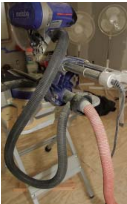
With the optional $40 dust-extraction adapter, the user can connect a vacuum to the miter saw and collect dust from inside the blade housing and from under the table.
