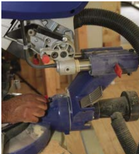
The author pulls a spring-loaded pin on the KGS 305 to disengage a bevel preset. The grooved silver piece to the right is a quick-acting lever that locks in the bevel. Unlike most bevel-lock mechanisms, this one is easy to reach from the front of the saw.
