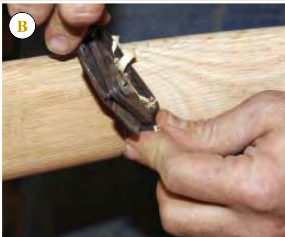
Figure 7. The author cleans up the joints in the handrail with a small plane (A), a spokeshave (B), and sandpaper (C).
