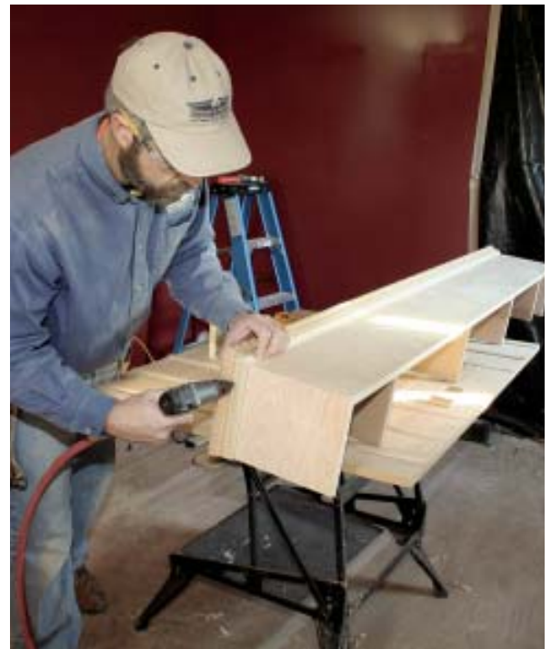
Figure 5. The mantelshelf begins as a plywood box, butt-jointed along the bottom edge and with the front and sides mitered together. A few cleats pocket-screwed inside reinforce the box (above); the butt joint is covered with molding (right).
