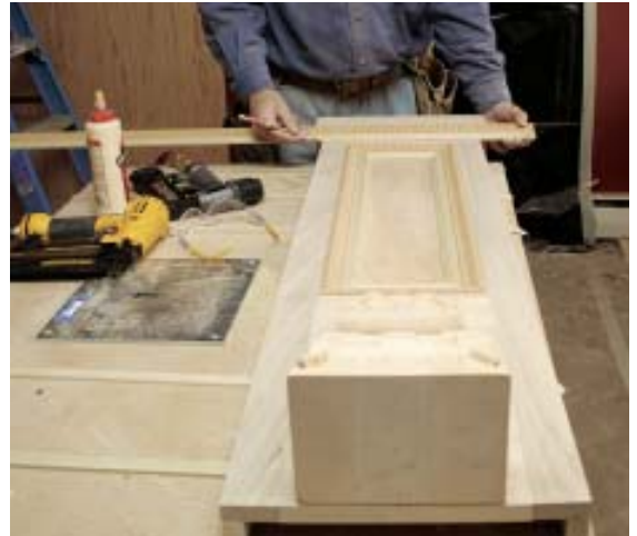
Figure 4. After applying glue and carefully positioning the corbels, the author pins each in place to make sure it won't move, then screws into it through the back of the panel for a strong connection (left). When installing the pilaster bases, he is careful to place the molding so that the repeating pattern turns the mitered corners symmetrically (above).
