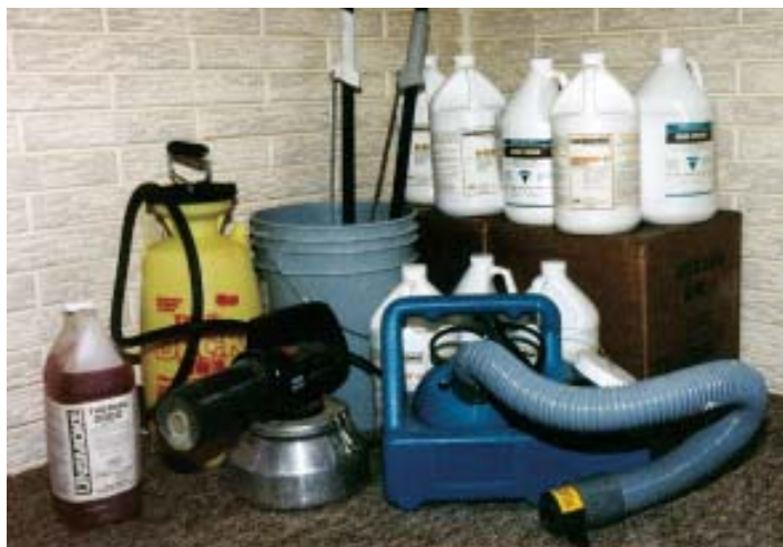
Figure 7. To control smoke odor, the author uses chemicals specifically formulated for cleaning and deodorizing. Some are simply applied by mop or brush, while others require specialized equipment, such as the thermal fogger (shown at left in photo) and wet fogger (shown at right).
