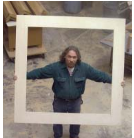
Figure 2. Cupola construction began with a one-piece bottom plate cut from 1/2-inch Baltic birch plywood.
