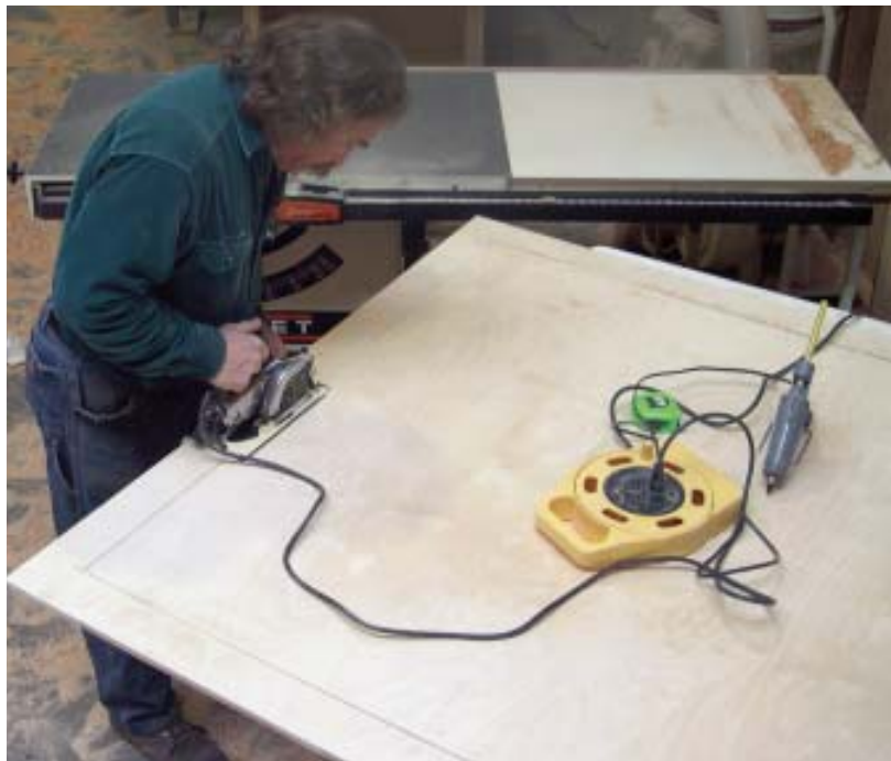
Figure 2. Cupola construction began with a one-piece bottom plate cut from 1/2-inch Baltic birch plywood.
