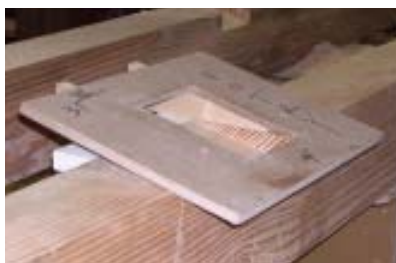
Figure 3. Top-bearing bits came in handy for following plywood and MDF templates — for cutting mortises (far left), for shaping a tenon on the end of a rafter tail (above), and for routing an angled pocket (left).
