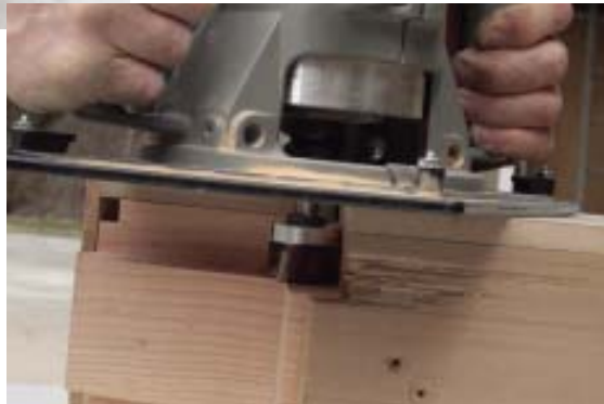
Figure 4. Two-sided “saddle” templates allowed the author to work from both sides of thick stock to cut a tenon using a top-bearing bit.
