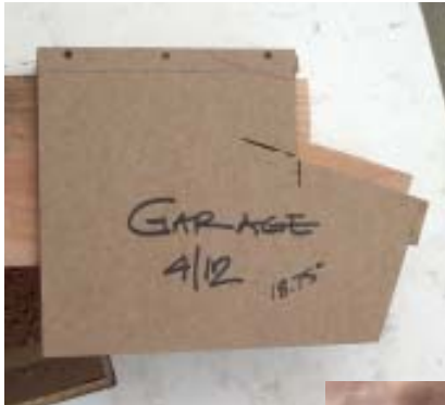
Figure 4. Two-sided “saddle” templates allowed the author to work from both sides of thick stock to cut a tenon using a top-bearing bit.
