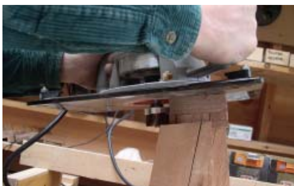
Figure 3. Top-bearing bits came in handy for following plywood and MDF templates — for cutting mortises (far left), for shaping a tenon on the end of a rafter tail (above), and for routing an angled pocket (left).
