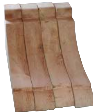
Figure 8. The giant knee brackets were cut out of large slabs, glued up from lengths of fir 6x8. The author used pieces cut from the same long beam and reversed the growth rings of every other one to cancel out the tendency of the wood to warp and cup.
