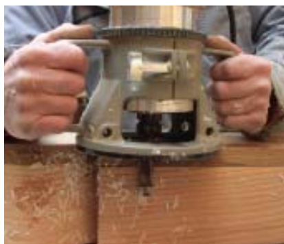
Figure 2. Following the shape of the band-sawn rafter tail, the author used a bottom-bearing bit (above) to profile the end of the attached rake frieze (right), which was glued to the tail with two-part epoxy. Once in place, the rake board looks like a full-dimension timber rafter (far right).
