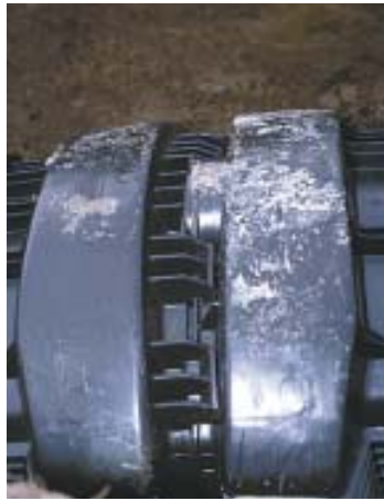
Figure 2. Chamber sections are designed to lock together easily. End caps are installed before placing the sections in the trench. They're molded with the pipe locations, so they can be used at either end of the trench. A couple of galvanized screws hold the end cap in place (right).
