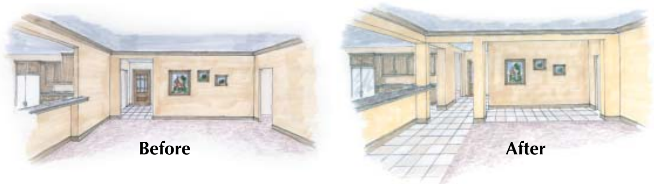
Figure 3. Two views from near the back door of the original and revised plans in Figure 2 highlight the effect of the added circulation galleries. In the original plan (left), it's difficult to tell where the circulation space ends and the family room begins. In the revised version (right), their separate functions are defined by the columns, header, and change of flooring; the added opening to the kitchen also improves traffic flow.
