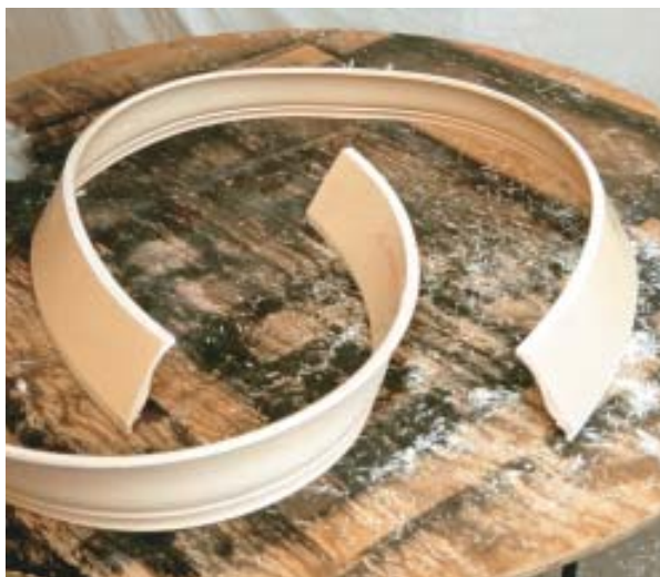
Figure 5. Crown molding can't be bent in place like baseboard, and there's little room for error when ordering. Manufacturers require a specific radius or template, and, although the material fits in a small box when shipped, it won't fit around a curve with a different radius.
