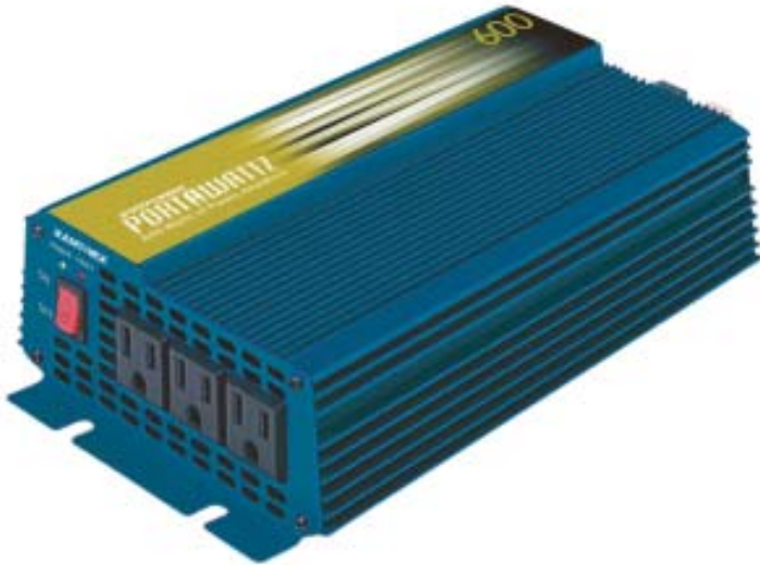
Figure 2. A 600-watt inverter mounted under the passenger seat converts the truck's 12-volt DC output into 120 AC for operating electronics, charging NiCad batteries, and occasionally powering drop lights and low-amperage power tools.
