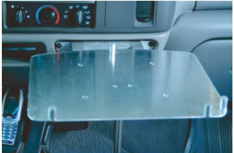
Figure 3. A computer table made from aluminum angle, bar stock, and \frac{3}{16} -inch plate is mounted in the dashboard cupholder slot and receives additional support from an aluminum rod that rests on the floor. The table can be locked to left, right, or center, making the author's laptop computer accessible from the passenger seat or — when the truck is parked — from the driver's seat.
