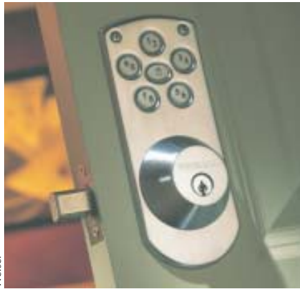
Figure 7. Although struggling for popular acceptance, electronic deadbolts provide keyless convenience for those in possession of a changeable, four- to eight-digit access code. A manual key override compensates for battery failure.
