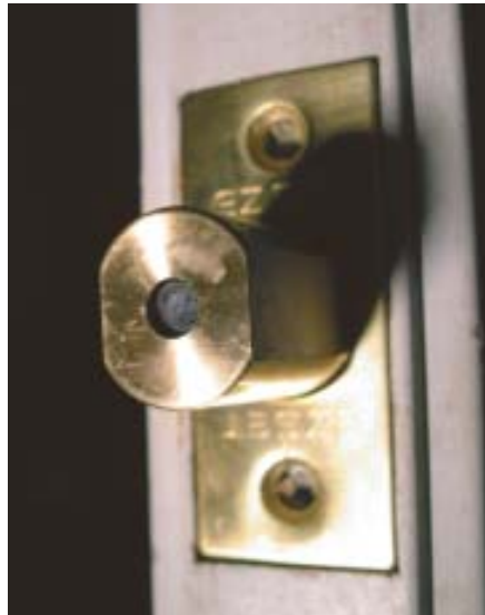
Figure 2. Hardened-steel reinforcement rods, inserted in the deadbolt, spin freely to frustrate hacksawing attempts.
