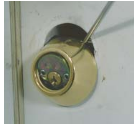
Figure 8. Hammering the deadbolt aside provides screwdriver access to retract the bolt. The bore diameter should be specific to the deadbolt cylinder, and the cylinder should insert into the bore to prevent dislocation.
