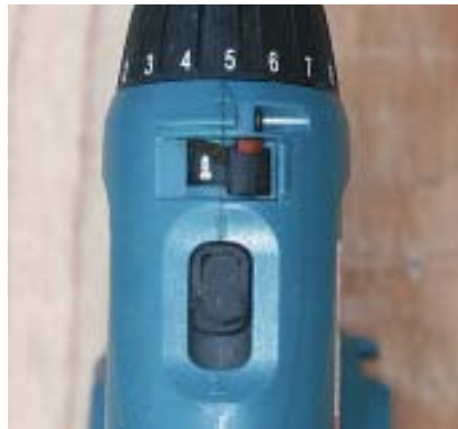
Figure 4. The Makita drill features a convenient top-mounted lever that allows switching from driver to drill and back without losing the dialed-in clutch setting.
