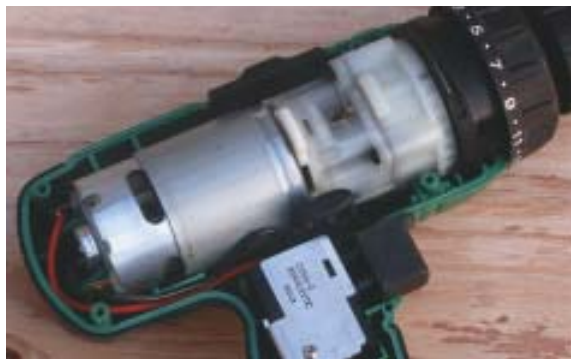
Figure 5. Most cordless drills, like the Hitachi (top), have can-style motors. The field, armature, fan, and brushes are encased in a metal housing and are typically serviced or replaced as a unit. The Makita drill (bottom) is built around an unusual two-piece motor equipped with a cooling fan.
