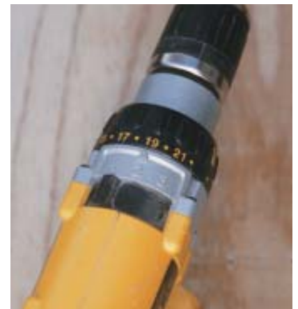
Figure 2. Most drill-drivers have two speed ranges; the DeWalt has three.
