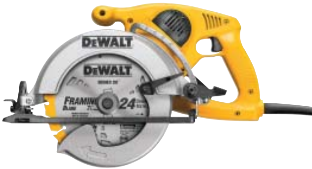
Figure 1. DeWalt’s inline offering, model 378, uses hypoid gearing instead of a traditional worm gear. Detractors claim that hypoid gears aren’t as durable, but advocates point out that they run quieter and the sealed gearbox means less maintenance.
