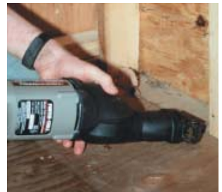
Figure 2. The gear housing's slight offset makes flush cutting easier. Rotating the bottom pivot 180 degrees allows you to cut equally well left or right.
