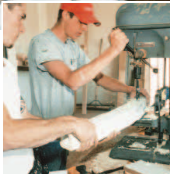
Figure 5. Balusters for the main railing were laid out on 5-inch centers (above). A hole saw in a drill press made for fast, accurate boring in the PVC radius railings (left) as well as the steel-reinforced straight rails.
