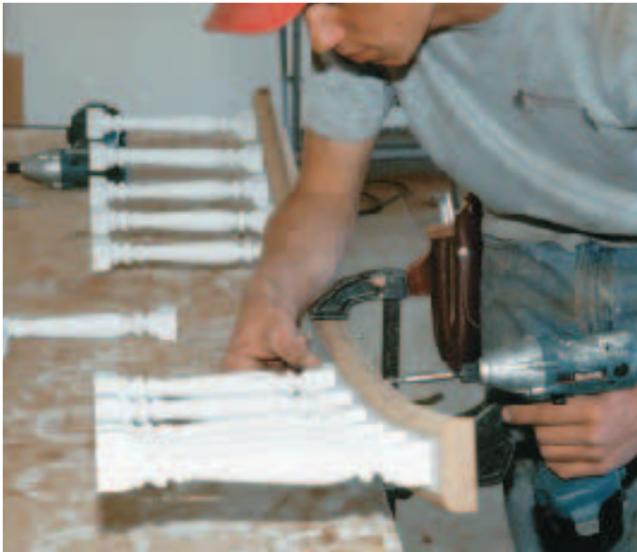
Figure 4. Holes for the galvanized screws were predrilled in both the rail and the spindles (left), but the Fypon adhesive provides the real strength for the spindle assemblies (right).
