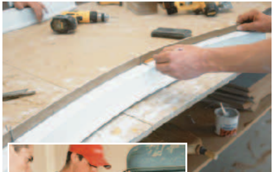
Figure 5. Balusters for the main railing were laid out on 5-inch centers (above). A hole saw in a drill press made for fast, accurate boring in the PVC radius railings (left) as well as the steel-reinforced straight rails.
