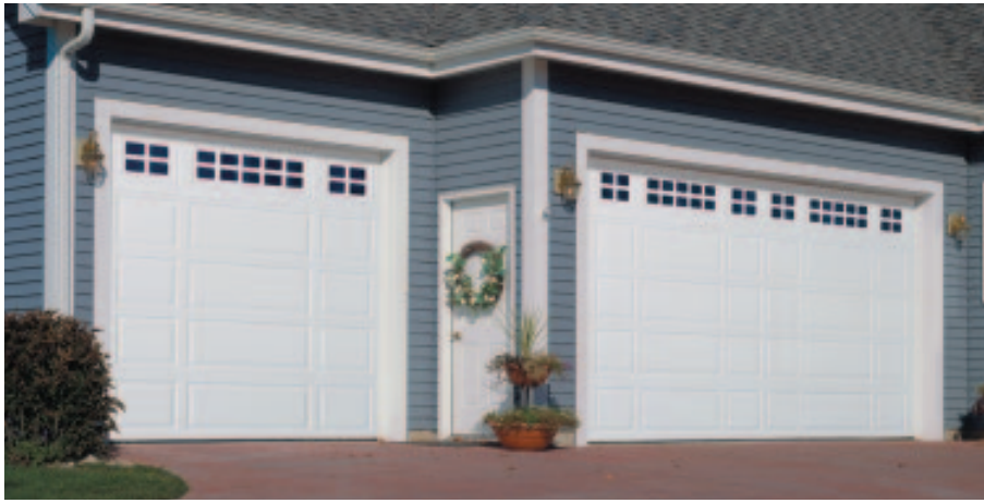
Figure 1. The new Relante steel door from Raynor is insulated with 1 3 / 8 inches of blown-in polyurethane foam. A single door sells for about $550 and is said to have an R-value of 12. The polyurethane is injected with a non-HCFC blowing agent that does not deplete atmospheric ozone.
