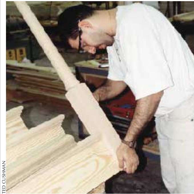
Figure 1. The stair shop prefits each railing system to the actual stairs as the stairs are built, so that no complicated layout is needed on site. Here, a shop carpenter test-fits a post to a stair set (left), then checks the plumb cut on a railing (right).
