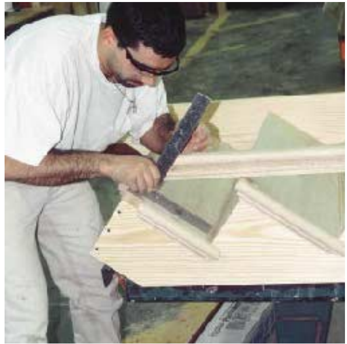
Figure 1. The stair shop prefits each railing system to the actual stairs as the stairs are built, so that no complicated layout is needed on site. Here, a shop carpenter test-fits a post to a stair set (left), then checks the plumb cut on a railing (right).
