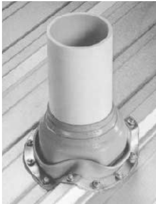
Figure 3. To seal round penetrations, use a special rubber boot jack with a moldable aluminum compression ring, like this one from ITW Buildex. The ring can be formed to fit almost any panel rib profile.
