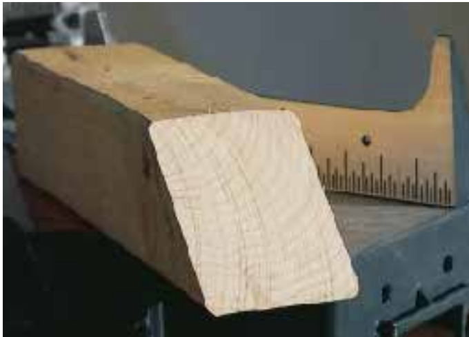
Figure 3. Here's what an unstable blade will do to the quality of your cut.
