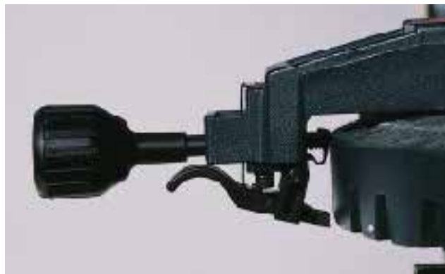
Figure 2. A miter detent override helps with adjustments close to the detent. When the override is disengaged the miter detents function; when engaged they do not.
