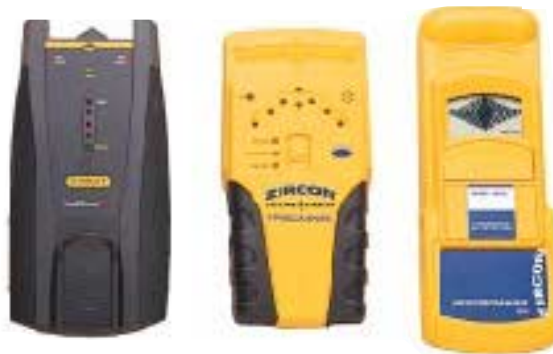
Figure 2. In the multi-function class, Zircon's Videoscanner and TriScanner performed noticeably better than Stanley's Intellisensor Pro.
