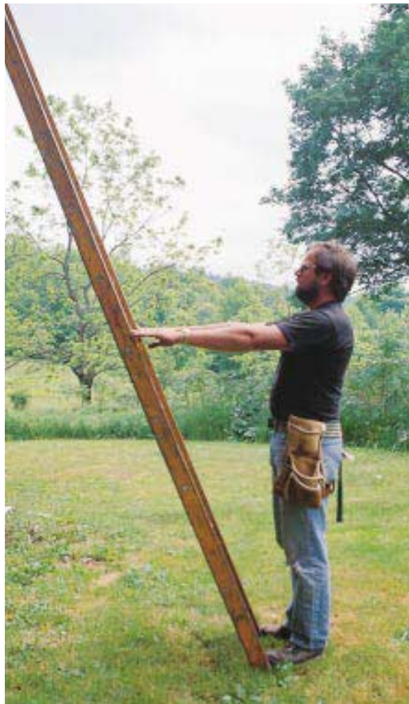
Figure 2. A quick way to find the proper angle for an extension ladder is to stand with your arms level and fully extended. Your fingertips and toes should just touch the rails of the ladder. The correct base/height ratio is 1 to 4.
