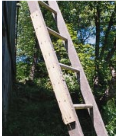
Figure 3. A shaky footing (upper left) is an accident waiting to happen. Dig out a level area and use a 2x10 pad. Driving a fastener through the ladder rail (upper right) weakens the rail and voids the manufacturer's warranty. Never use a ladder in a horizontal position (bottom left): You'll weaken the connections between the rungs and the rails, void the manufacturer's warranty, and risk an OSHA fine. Don't make creative repairs (bottom right) — you'll be assuming all the liability if the ladder fails. Instead, you should destroy the ladder.
