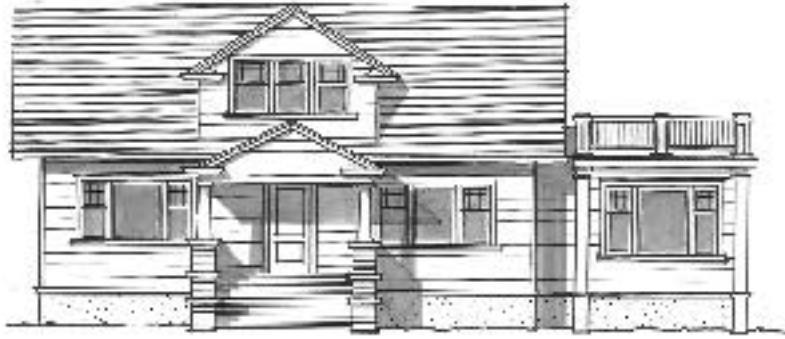
Figure 3. In the end, the author and client decided on a flat roof. The addition uses the same siding and trim as the existing house, while the railing on top and the 3-foot-wide reveal between house and addition let the addition stand comfortably beside the main house despite its lack of a pitched roof.
