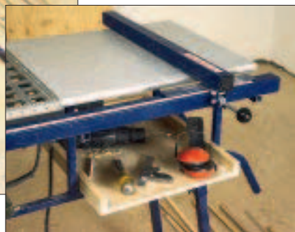
Trojan's folding table saw stand holds an 8 1 / 4 -inch table saw at a comfortable 36-inch working height and increases the rip capacity from 12 inches to 28 inches (left). The rugged frame, which supports an upgraded fence, can accommodate a handy site-made shelf (below).
