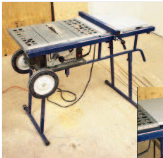
Trojan's folding table saw stand holds an 8 1 / 4 -inch table saw at a comfortable 36-inch working height and increases the rip capacity from 12 inches to 28 inches (left). The rugged frame, which supports an upgraded fence, can accommodate a handy site-made shelf (below).
