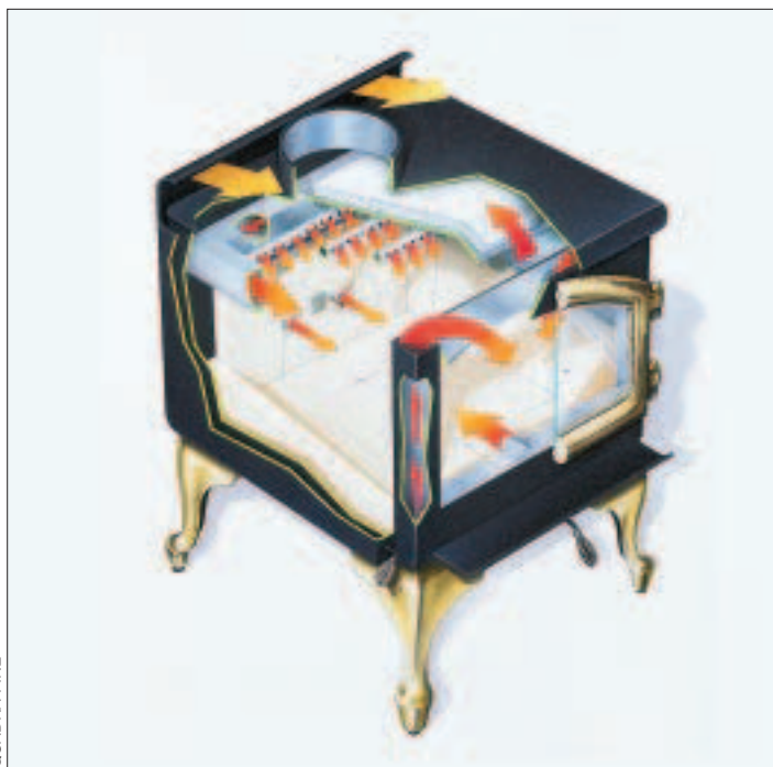
Figure 1. This noncatalytic wood stove uses ceramic insulation and a lining of firebrick to help maintain high combustion temperatures. Air is channeled to several parts of the firebox to ensure complete burning of gases.
