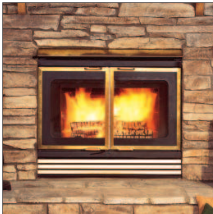
Figure 2. Unlike ordinary zero-clearance fireplaces, this fireplace insert passes EPA Phase II standards for clean combustion. Built-in blowers on fireplace inserts boost the heat output to equal or exceed that of freestanding stoves.
