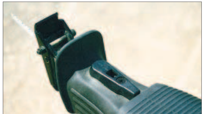
The easiest shoe adjustments are made with a lever like the one on this Makita JR3020. Simply swing it 90 degrees, set the shoe in a new position, and swing the lever back. Milwaukee's Super Sawzall has a similar lever.
