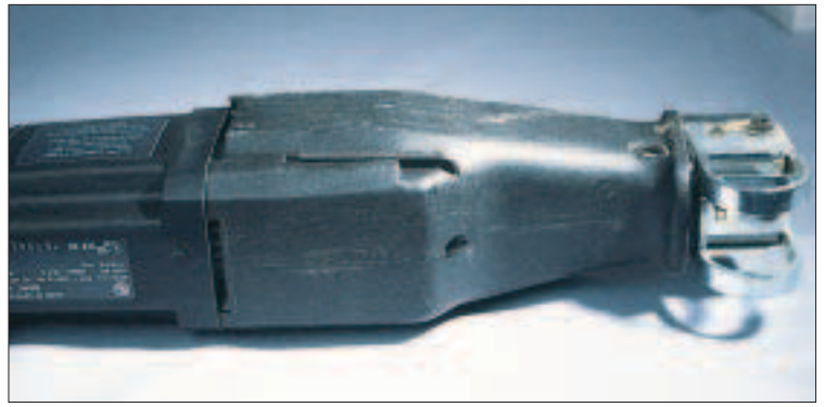
Porter-Cable's new 737 Tiger Saw has the first keyless blade clamp on a recip saw (left). A twist of the knurled cylinder in the direction of the arrow opens up the slot, enabling you to slip a blade in or out. Other manufacturers have tried to make the hex wrench more accessible: Both Milwaukee's Super Sawzall and AEG's SSPE 800 (right) have a storage slot on the boot of the tool.
