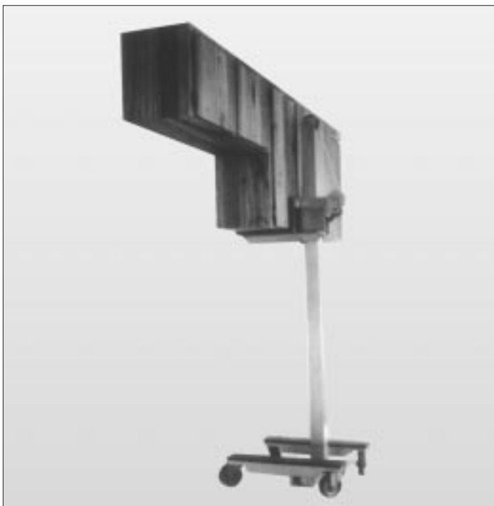
Figure 1. A cabinet hoist, like this one by Gil Lift, lets a carpenter install upper cabinets without a helper. It's also handy for moving cabinets and other bulky items around the site.
