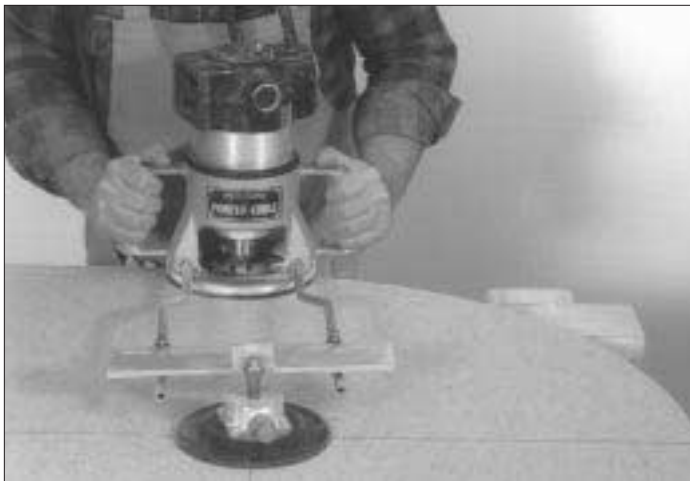
Figure 2. The Air Compass was designed for routing curves in solid-surface countertops, but it's also great for general-purpose router work. No screws or fasteners are needed — the suction cup grabs onto any flat surface.
