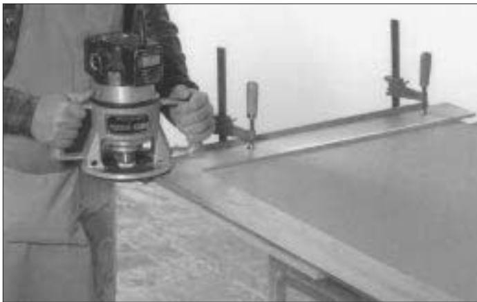
Figure 3. Specialty router guides are thicker, more precise, and less likely to bend under pressure than site-made straightedges or the standard carpenter's variety.
