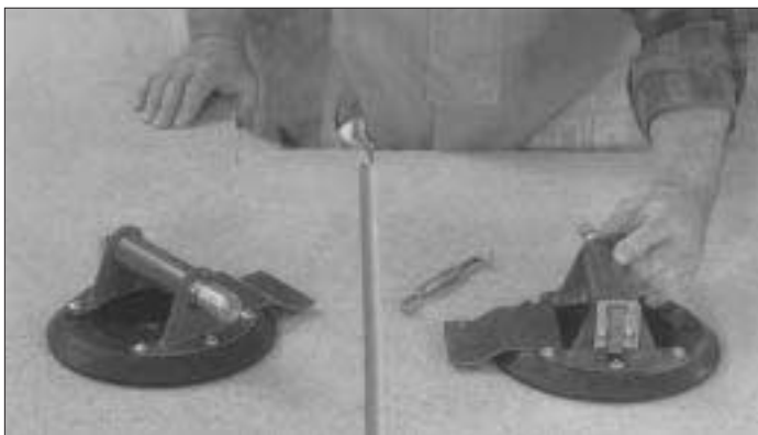
Figure 4. The Power Grip system consists of a pair of suction cups and a turnbuckle. It's good for drawing countertops, cabinets, or any other flat surfaces together.
