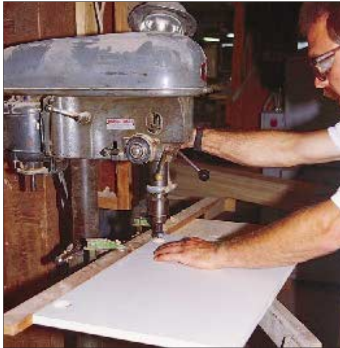
Figure 3. A drill press and a special 35mm bit are essential for mounting cup hinges.
