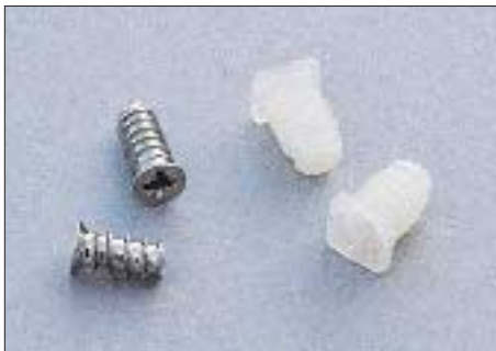
Figure 4. Specialty mounting screws. In particleboard substrates, large-diameter euro screws, at left, help prevent stripping of the screw hole. An option that works even better is a friction-fit nylon insert, at right, which accepts a #6 wood screw.
