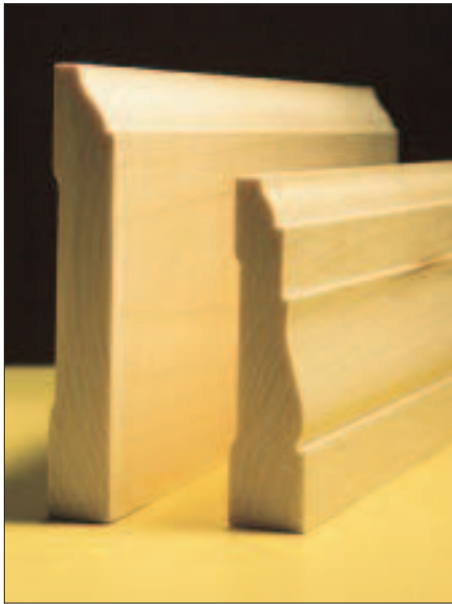
Figure 2. AWI specifies that all Custom and Premium trim stocks have a hollow on their back side. Called “backing out,” this helps the trim lie flat over irregular surfaces and lessens the chance that it will cup and withdraw the fasteners.
