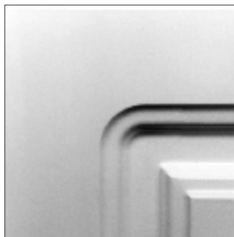
Figure 4. Over time, white painted hardwood cabinets tend to show small cracks at the joints (top). An alternative is to use a foil-wrapped MDF front (above).
