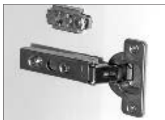
Figure 6. Fully concealed cup hinges are adjustable in three dimensions, making it easier to keep full overlay doors aligned. Many cup hinges allow you to remove the door by unclipping the hinge body from the base plate (above).
