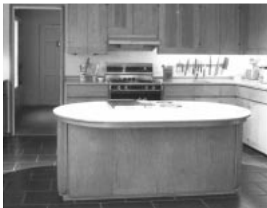
Figure 2. A countertop wider than 42 inches should have curved or angled corners to make it easier to reach the entire work surface from all sides.
